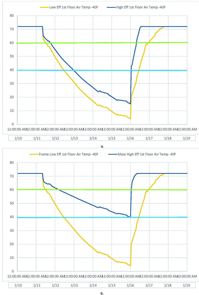
Figure 11 Comparison of a high efficiency versus a low efficiency and typical 1980 in building heating failure results at -40^{\circ}\text{F} ( -40.0^{\circ}\text{C} ) weather for a (a) frame building and a (b) mass building.
