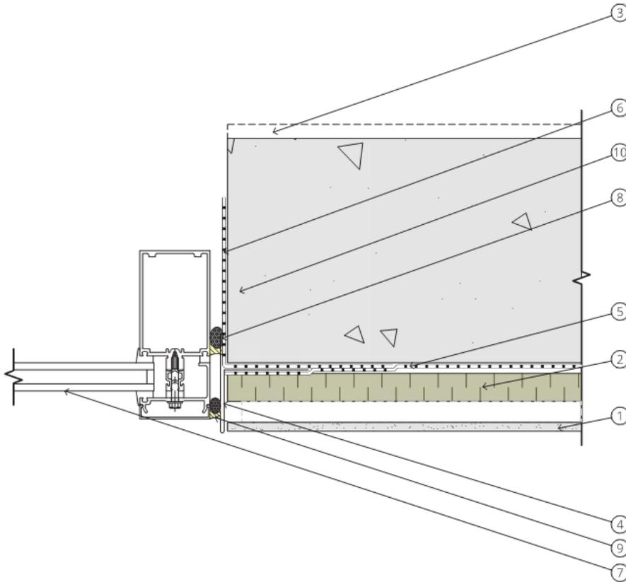
1. Cladding as per architectural – rain shedding layer for water control
