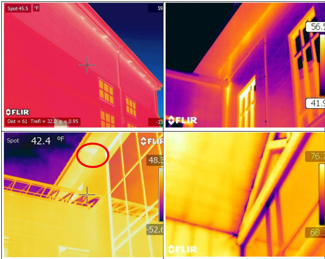
Figure 4-1. Examples of air leakage observed at soffit transition: from outside (top left, top right, bottom left), and from interior (bottom right).
