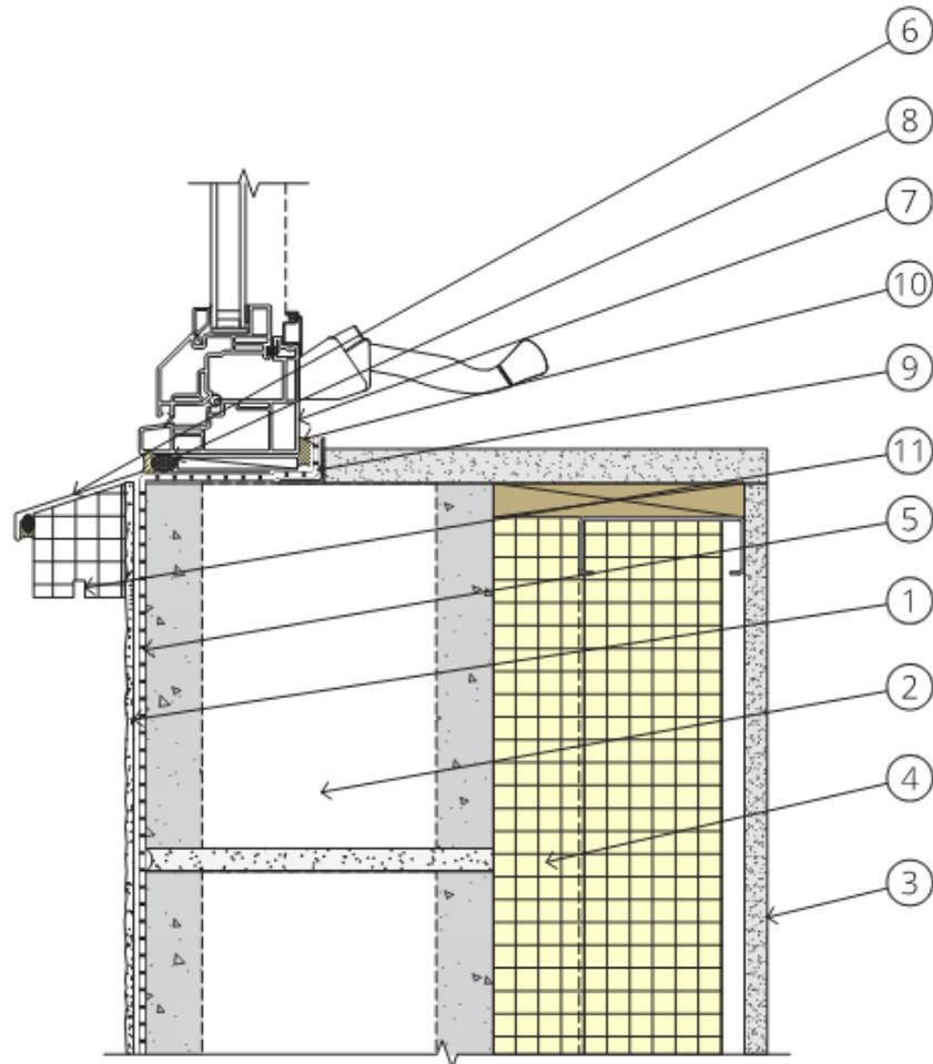
1. Cladding as per architectural - drained and vented cladding is recommended (water shedding layer)
