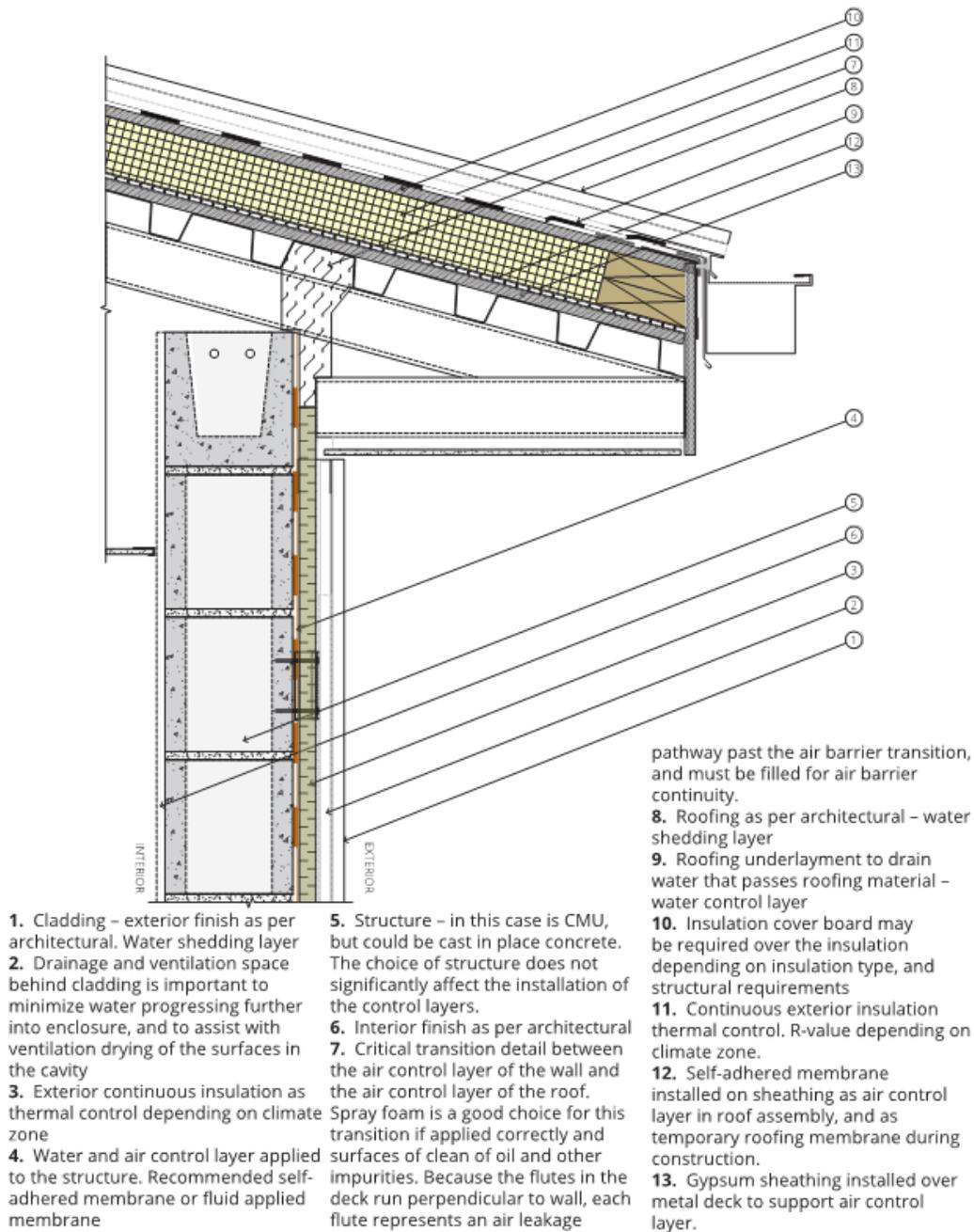
**Figure 4-30. Sloped unvented roof assembly with overhang.**
