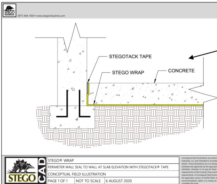
**Recommend installing vapor barrier to foundation wall.**
