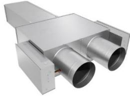
**Figure 5-15. A dual-duct VAV terminal unit can be used for control of both cooling air and air from the DOAS.**
