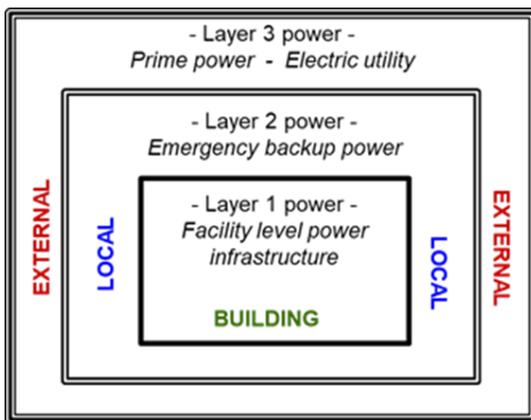
**Figure 3-1. Layers of energy supply to mission-critical facilities.**
