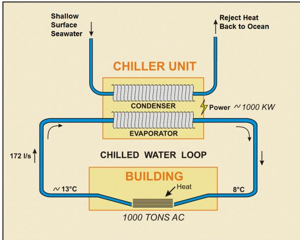
**Figure 6-3. Schematic of a shallow water-cooled chiller unit.**
