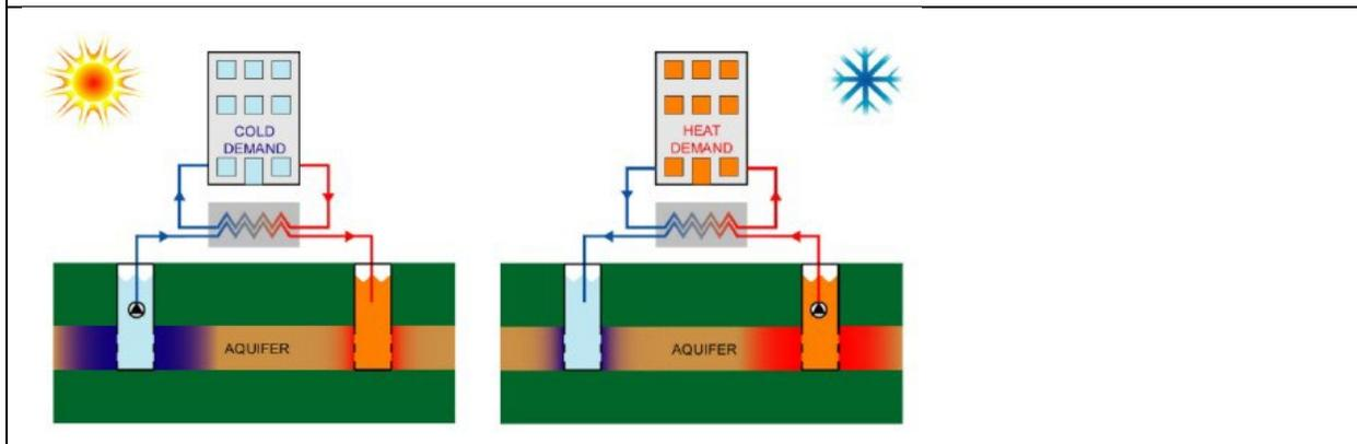
**Open-loop Ates system scheme with the seasonable reversible operation. In summer, aquifer water is extracted from the cold well (left) and injected into the warm well (right). Free cooling (through a heat exchanger) or additional Ground Water Heat Pump (GWHP) (cooling mode) is used for cooling. During the winter period, the operation is reversed using GWHP for heating (Drijvert et al. 2001)**
