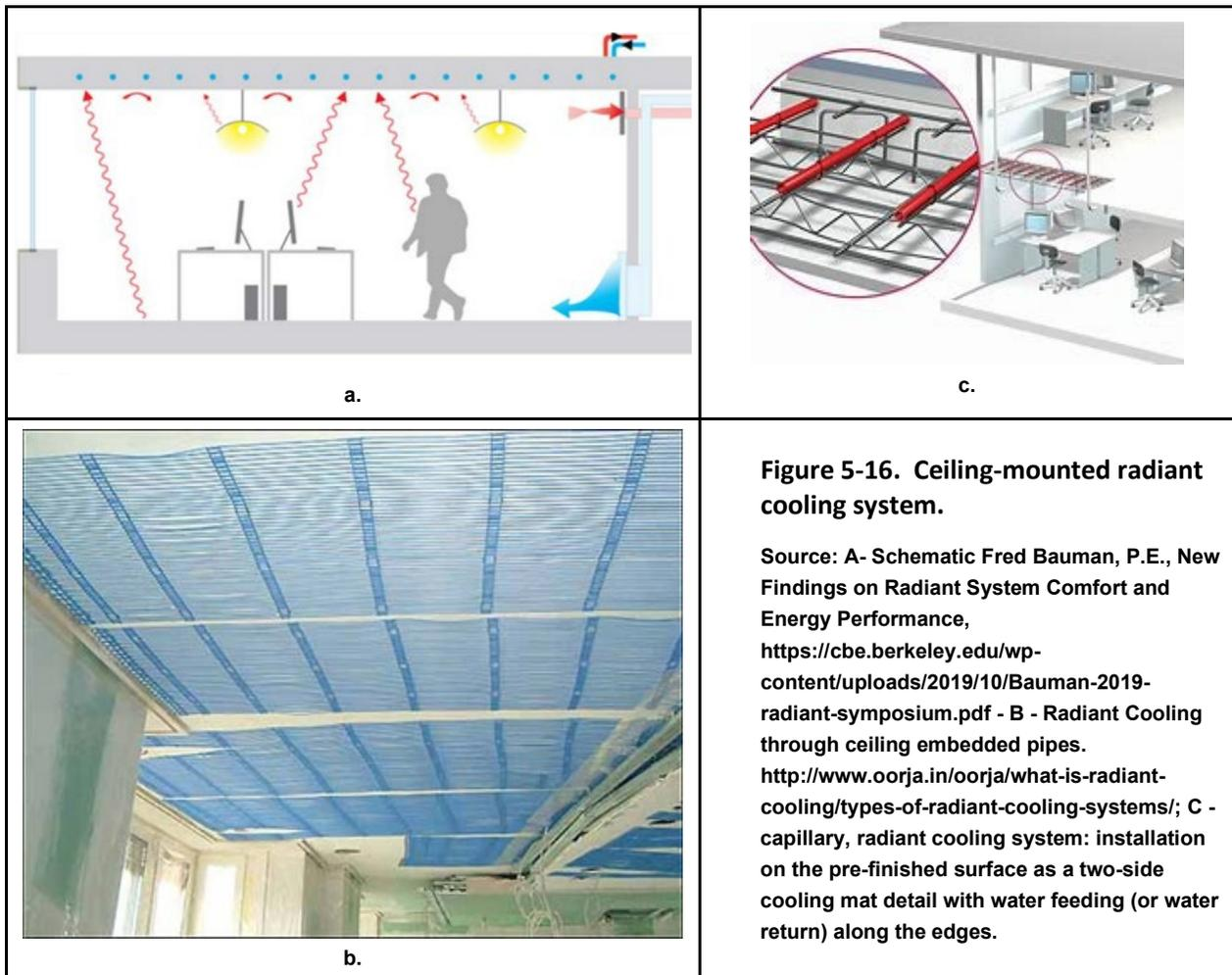
**Figure 5-16. Ceiling-mounted radiant cooling system.**
