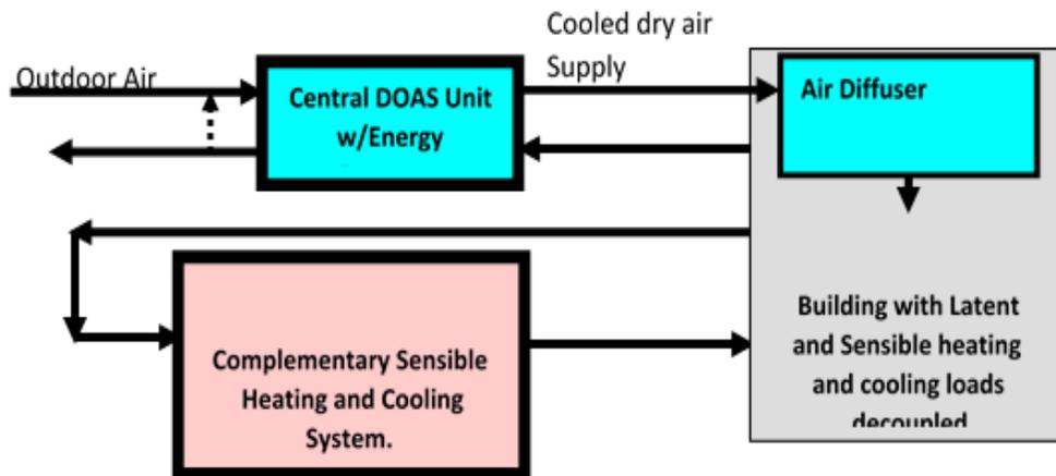
**Figure C-1. Basic DOAS schematic with exhaust energy recovery.**
