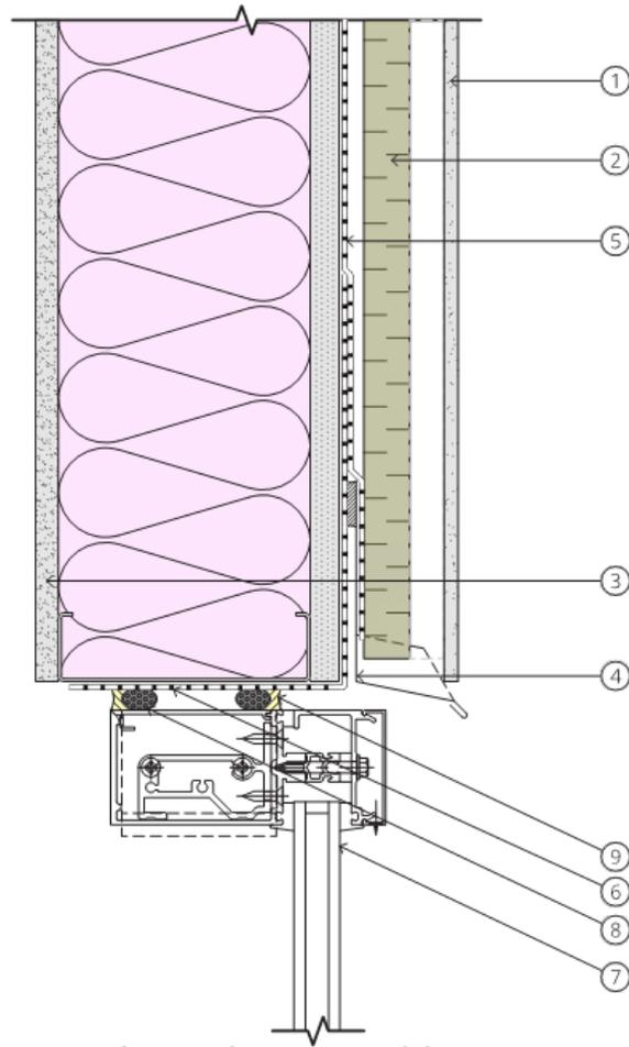
1. Cladding as per architectural – rain shedding layer for water control
