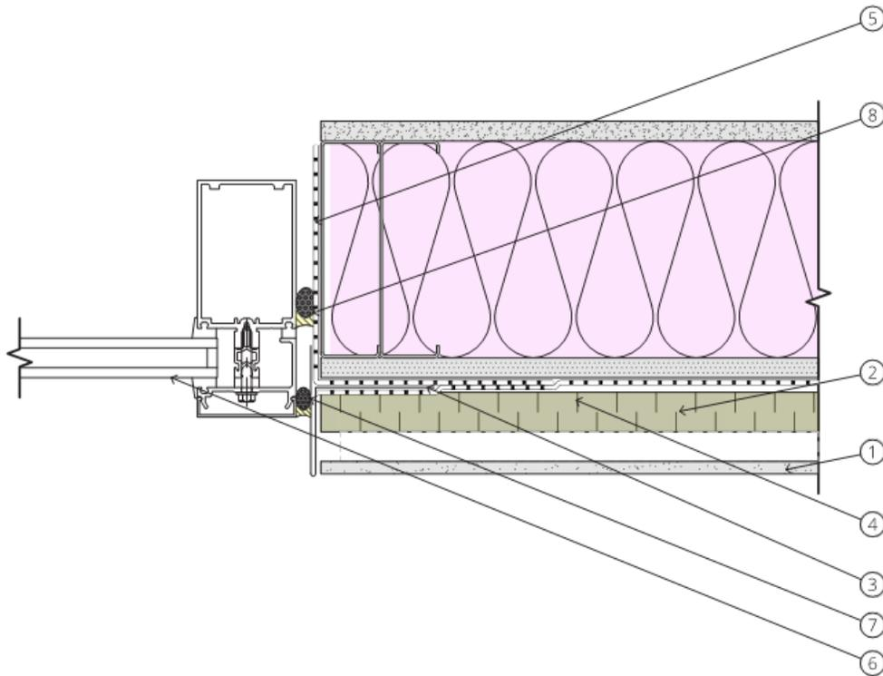
1. Cladding as per architectural – rain shedding layer for water control
