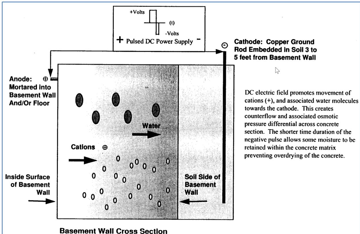
Figure 4-16. Schematic diagram of the EOP system.
