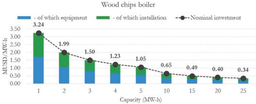
**Fig. F.39** Nominal investment by capacity for a wood chips boiler
