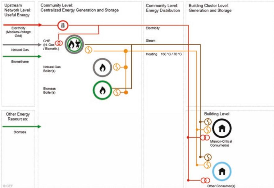
Fig. 7.15 Schematic of the energy system at the University of British Columbia (CAN)
