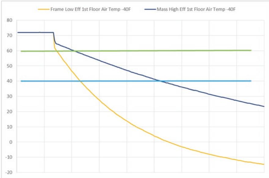
**Fig. 5.19** Comparison of indoor air temperature decay in low-efficiency frame building vs. high-efficiency mass building with a heating system failure at outdoor air temperature of  $-40^{\circ}\text{F}$  ( $-40^{\circ}\text{C}$ )
