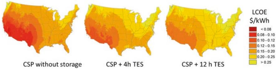
**Fig. G.4** LCOE across the CONUS for concentrating solar power systems including 4 hours and 12 hours of TES. Costs in sunny areas are on the order of \$0.08/kWh without storage and up to \$0.25/kWh in less sunny areas with 12 hours of thermal energy storage
