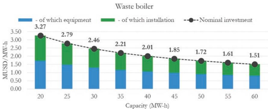
**Fig. F.42** Nominal investment by capacity for a waste boiler
