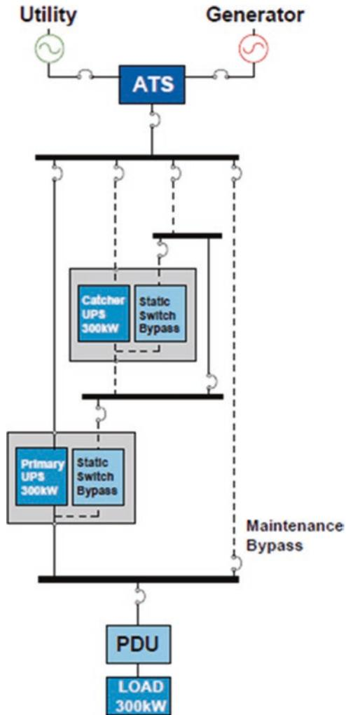
The secondary UPS can also be used to extend the run time of the primary UPS, switching from primary to secondary as the power delivery of the primary is consumed. Additional UPS capability is available for unexpected generator shutdown.
