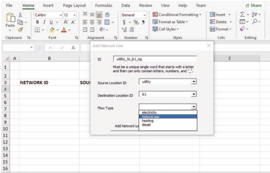
Fig. H.25 Adding a network link from utility to b1
