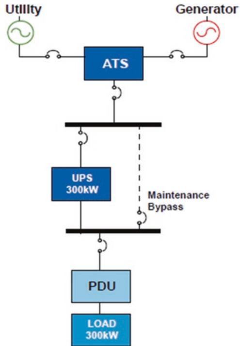
Most “ $N$ ” system configurations, especially under 100 kW, are placed in buildings with no particular concern for the configuration of the overall electrical systems in the building. In general, building electrical systems are designed with an “ $N$ ” configuration, so an “ $N$ ” UPS configuration requires nothing more than that to feed it. A common single module UPS system configuration is shown in Fig. C.2.
