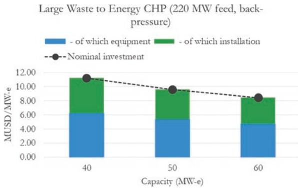
**Fig. F.14** Nominal investment for a large waste-to-energy CHP (220 MW feed, back-pressure)
