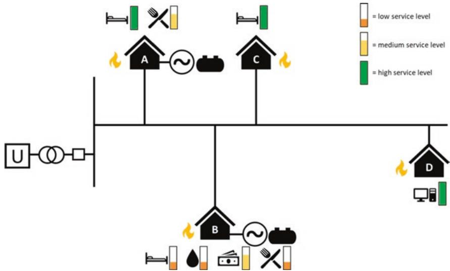
**Fig. 5.14** Critical functions and their service levels applied to the notional system. (Jeffers et al. 2020)
