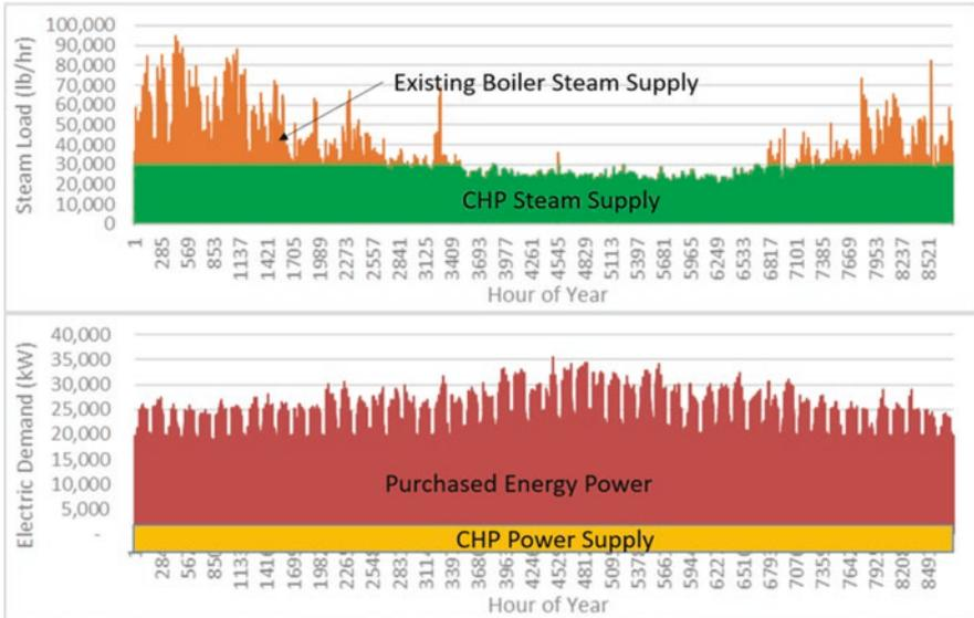
**Fig. I.3** CHP resilient solutions generate savings for an ESPC by offsetting heat (steam) and electrical purchases
