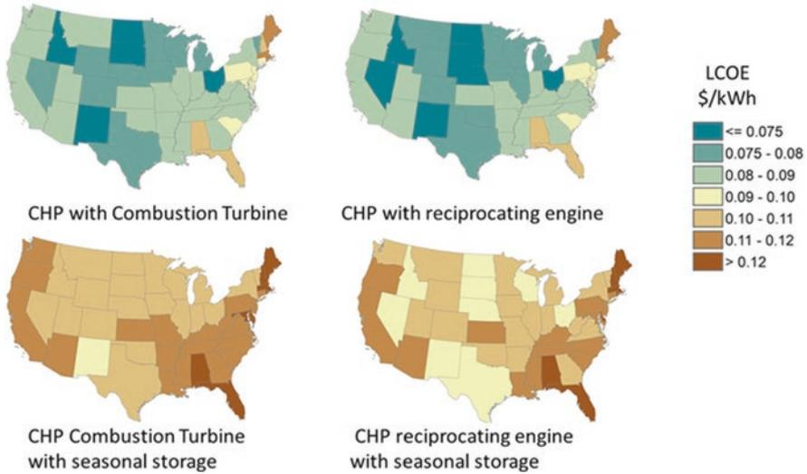
**Fig. 7.3** Levelized cost of energy (LCOE) across the CONUS based on 2018 natural gas prices for CHP systems based on combustion turbine and reciprocating engine and with/without seasonal thermal storage
