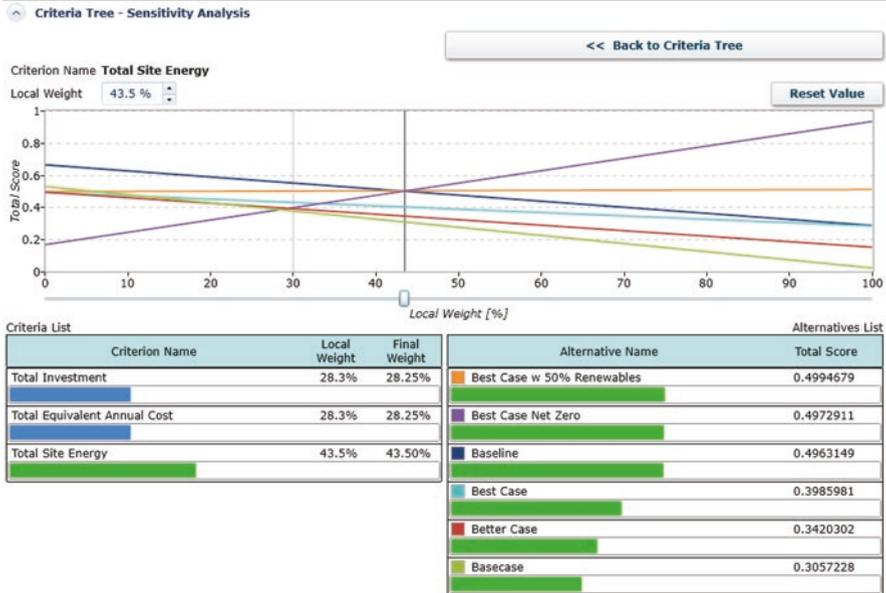
Fig. 9.6 Sensitivity analysis can be conducted on the criteria weights by moving the slider bar
