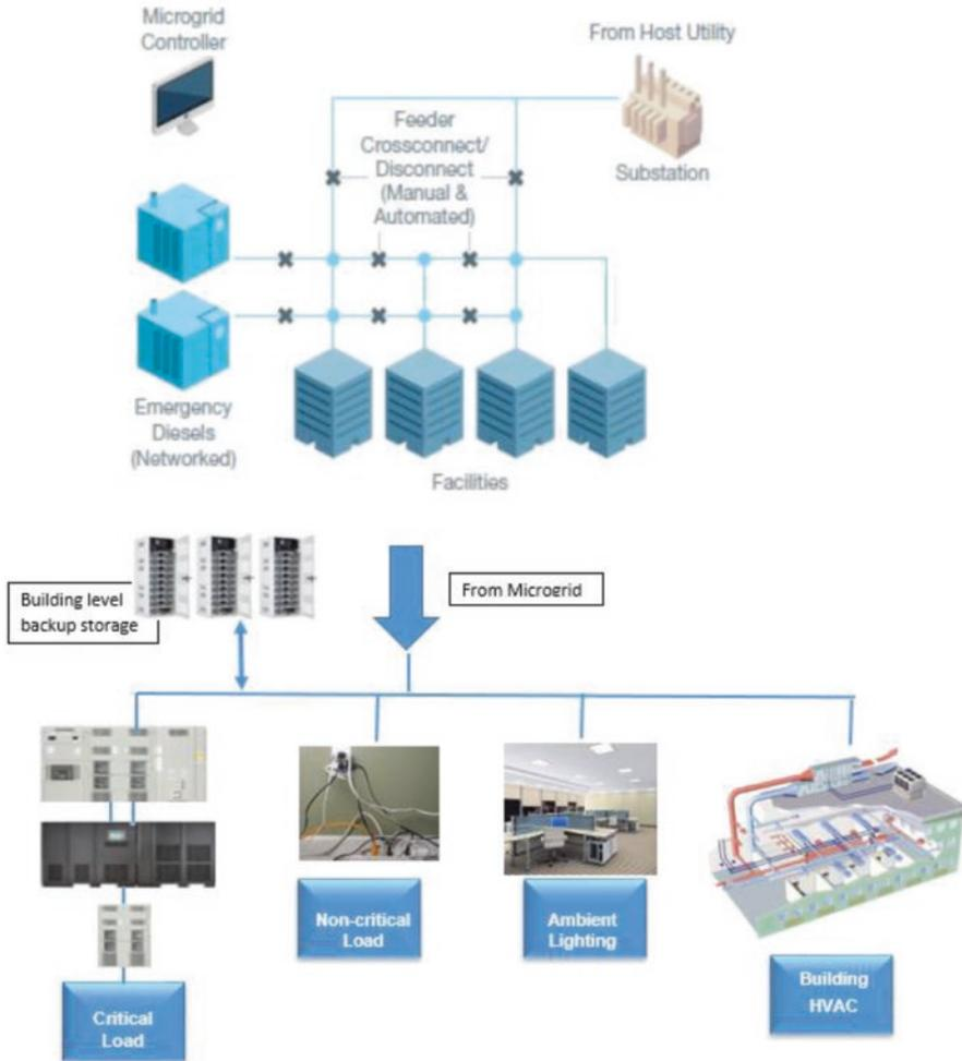
**Fig. F.15** Microgrid with centralized emergency generators and a building-level backup
