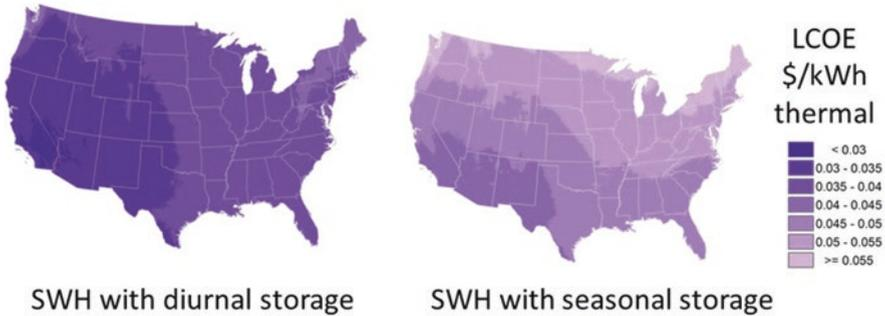
**Fig. G.7** LCOE of solar water heating systems varies from less than \$0.03/kWh in the best parts of the sunny Southwest to over \$0.055 in the Northeast and western Washington state
