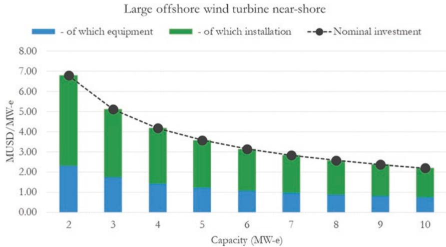
Fig. F.25 Nominal investment for large offshore wind turbine nearshore
