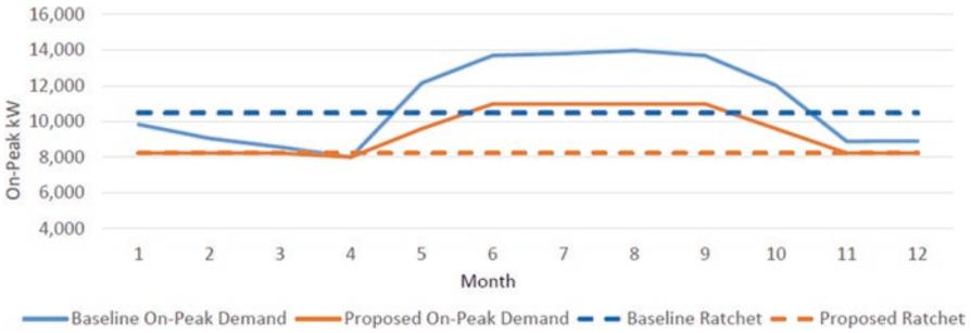
**Fig. I.1** Resilient ECMs can use their DERs to lower peak demand and ratchet charges to significantly save energy and provide savings in an ESPC
