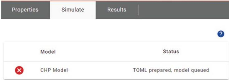
**Fig. 8.20** The ERIN simulation control panel in SMPL. This panel allows the user to start and stop the ERIN simulation(s), as well as provide status updates
