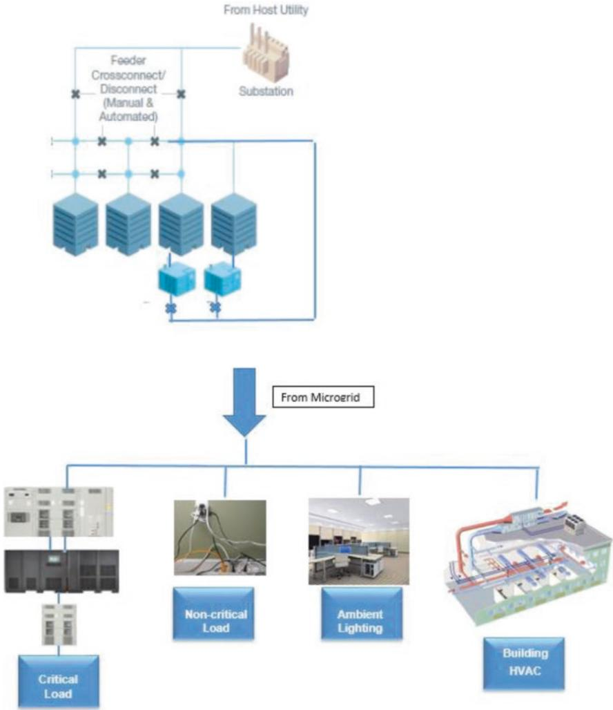
Fig. F.21 Microgrid with decentralized emergency generators
