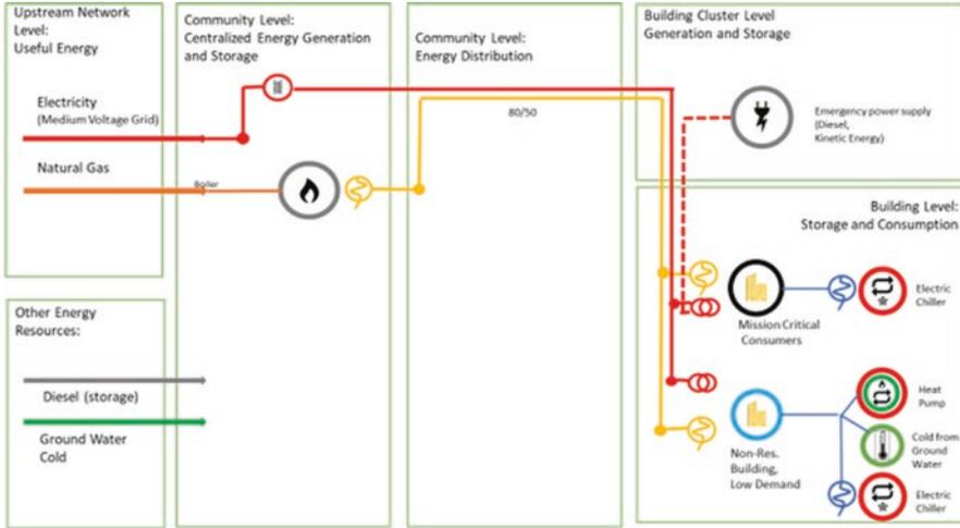
**Fig. B.5** Energy system architecture of the University Campus Technik in Innsbruck (AUT). The system is of type 1.3.4
