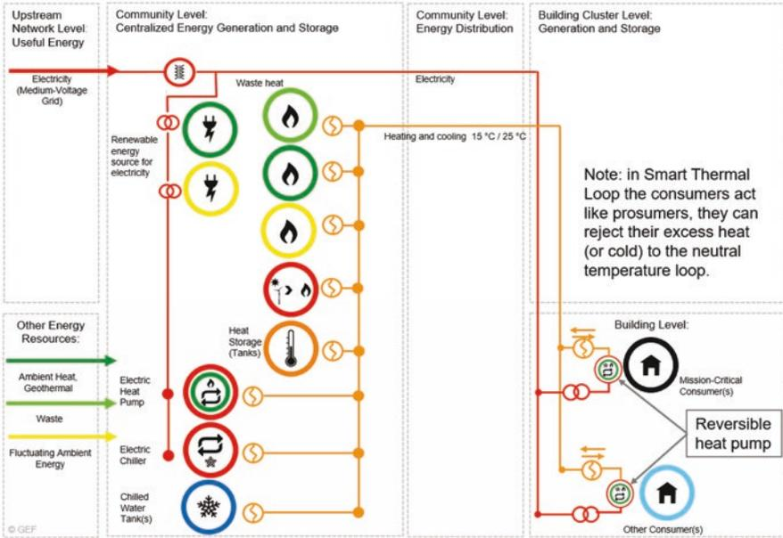
Fig. 7.21 Smart thermal loop, Melbourne (AUS)
