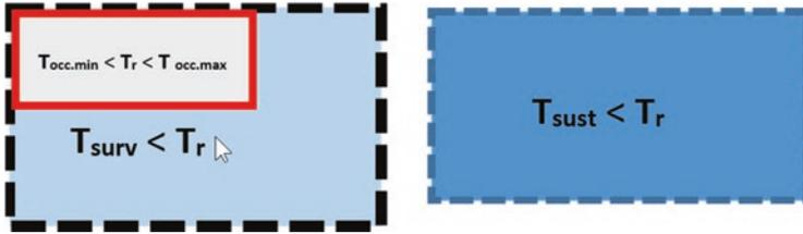
Fig. 5.20 Temperature reduction concept in mission-critical and non-mission-critical areas/buildings
