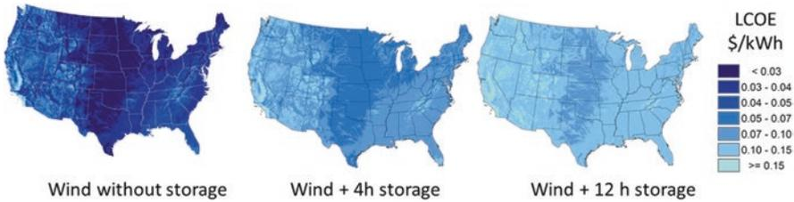
**Fig. G.5** LCOE across the CONUS for wind energy systems, including with 4 hours and 12 hours of battery storage. Costs vary from \$0.03/kWh in windy areas (Great Plains states of ND, SD NE, OK, TX) and as high as \$0.15/kWh in less windy areas with 12 h of battery storage
