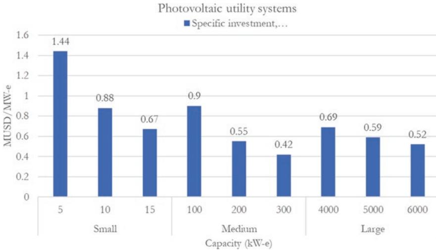
**Fig. F.22** Nominal investment for a small, medium, and large residential photovoltaic system
