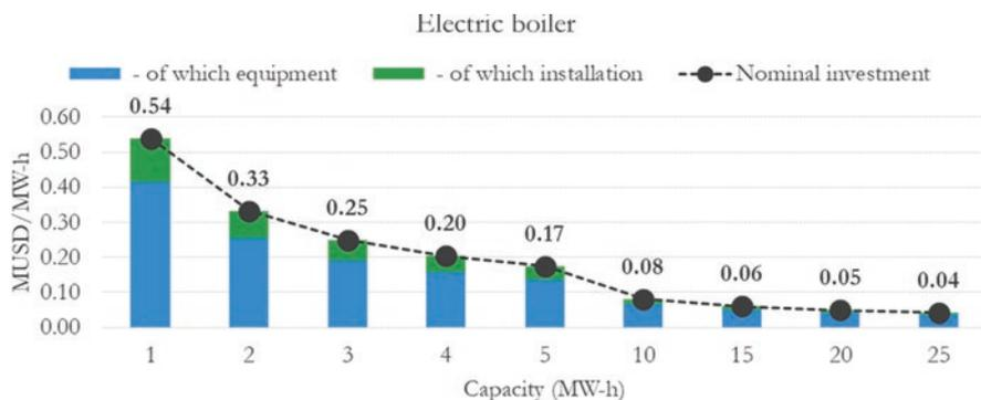
Fig. F.41 Nominal investment by capacity for an electric boiler
