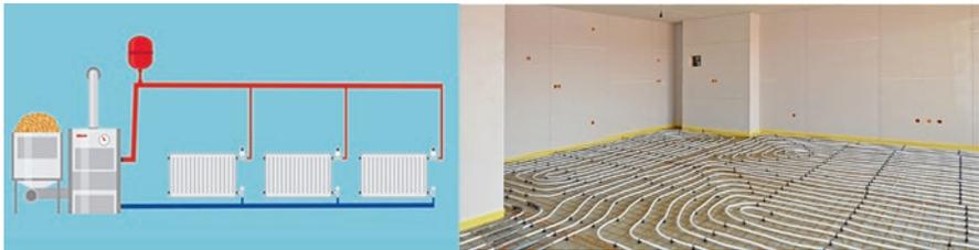
Fig. F.67 Central heating principle and floor heating
