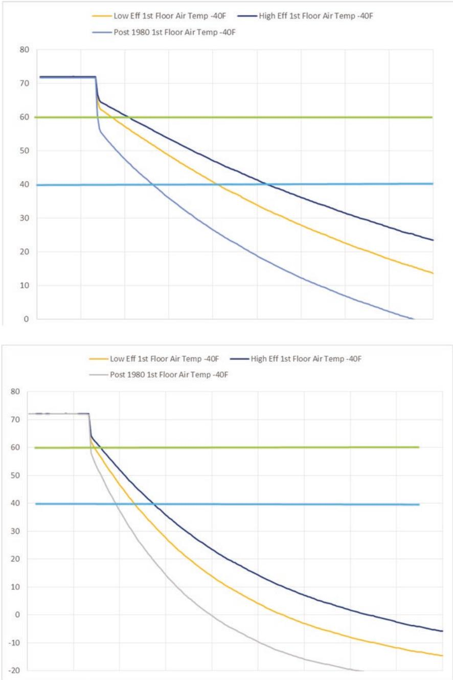
**Fig. 5.18** Indoor air temperature decay in high-efficiency, low-efficiency, and post-1980 buildings with a heating system failure at outdoor air temperature of  $-40\text{ }^{\circ}\text{F}$  ( $-40\text{ }^{\circ}\text{C}$ ): (a) mass building, (b) frame building
