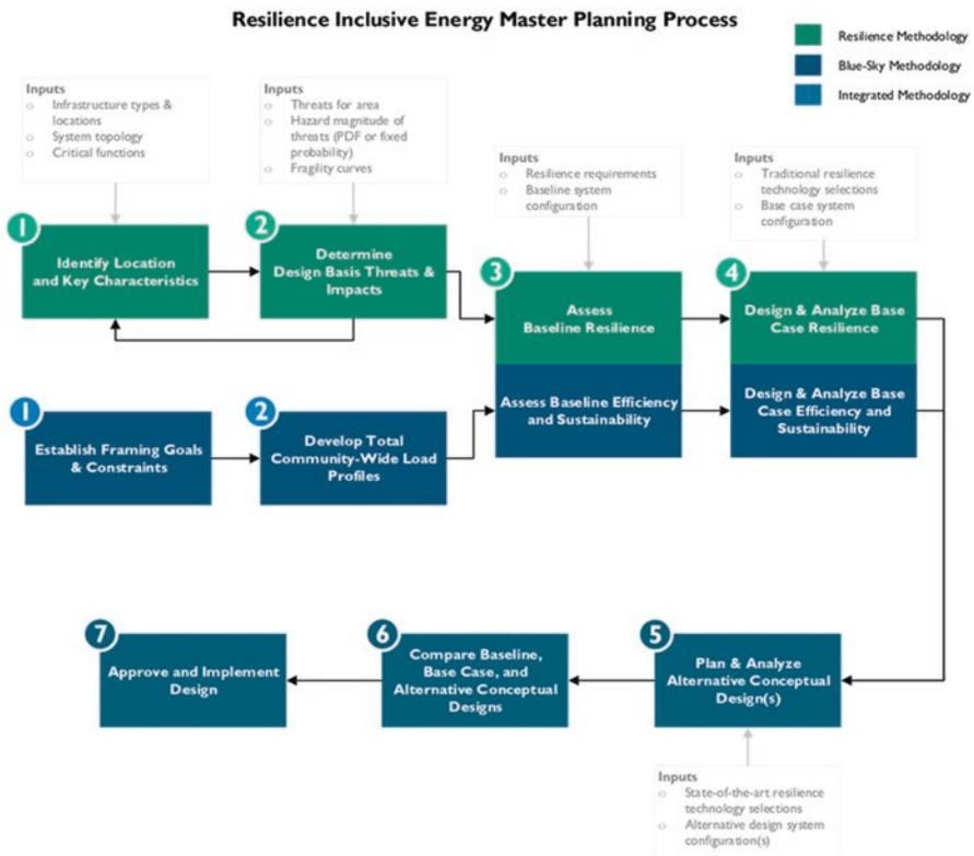
Fig. 3.1 Integration of Energy Systems Resilience Analysis into Energy Master Plan
