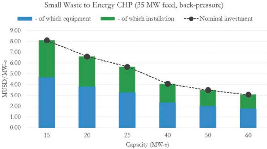
**Fig. F.12** Nominal investment for a small waste-to-energy CHP (35 MW feed, back-pressure)
