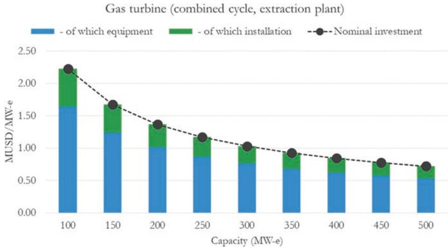
Fig. F.4 Nominal investment for gas turbine (combined cycle, extraction plant)
