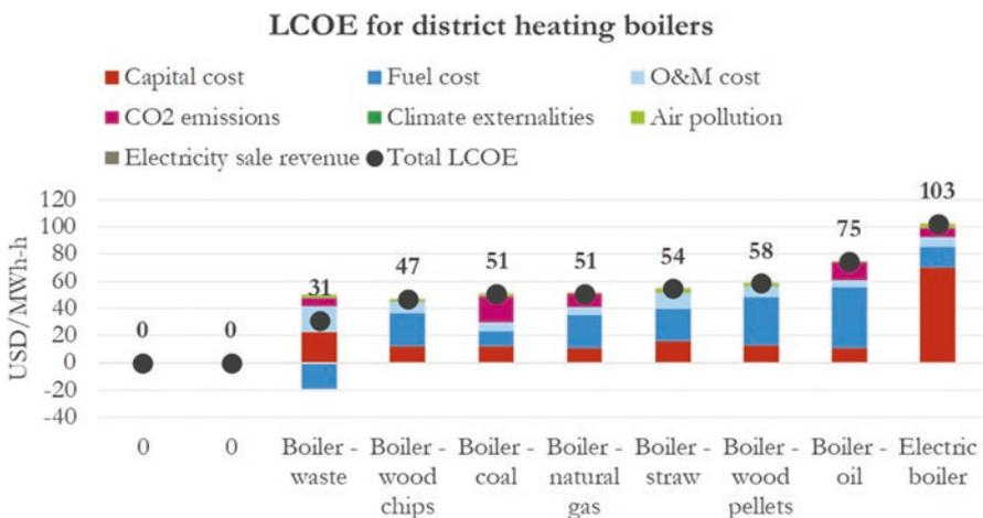
Fig. F.34 LCOE for district heating boilers
