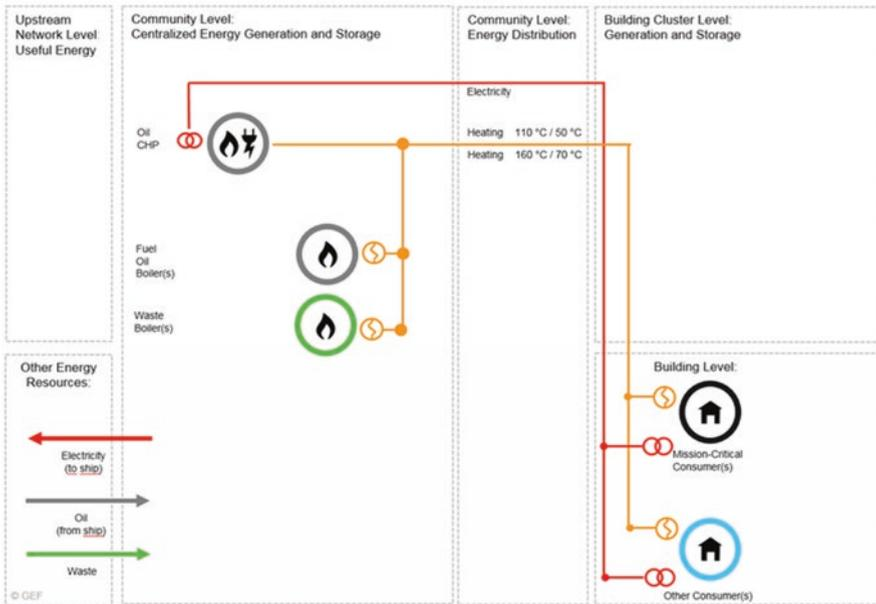
Fig. B.2 Energy system architecture for case study on Qaanaaq, Greenland
