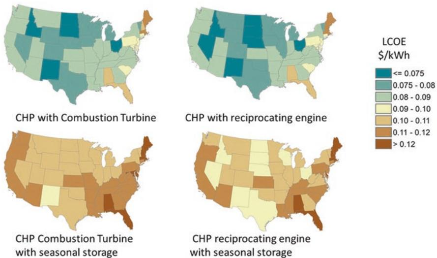
**Fig. G.6** LCOE across the CONUS based on 2018 natural gas prices for combustion turbine combined heat and power systems based on combustion turbine and reciprocating engine and with/without seasonal thermal storage. Costs vary from less than \$0.075/kWh in Western states where natural gas is least expensive and over \$0.11/kWh in states with higher gas costs in the Northeast. With seasonal storage, the cost varies from \$0.09/kWh to over \$0.12/kWh
