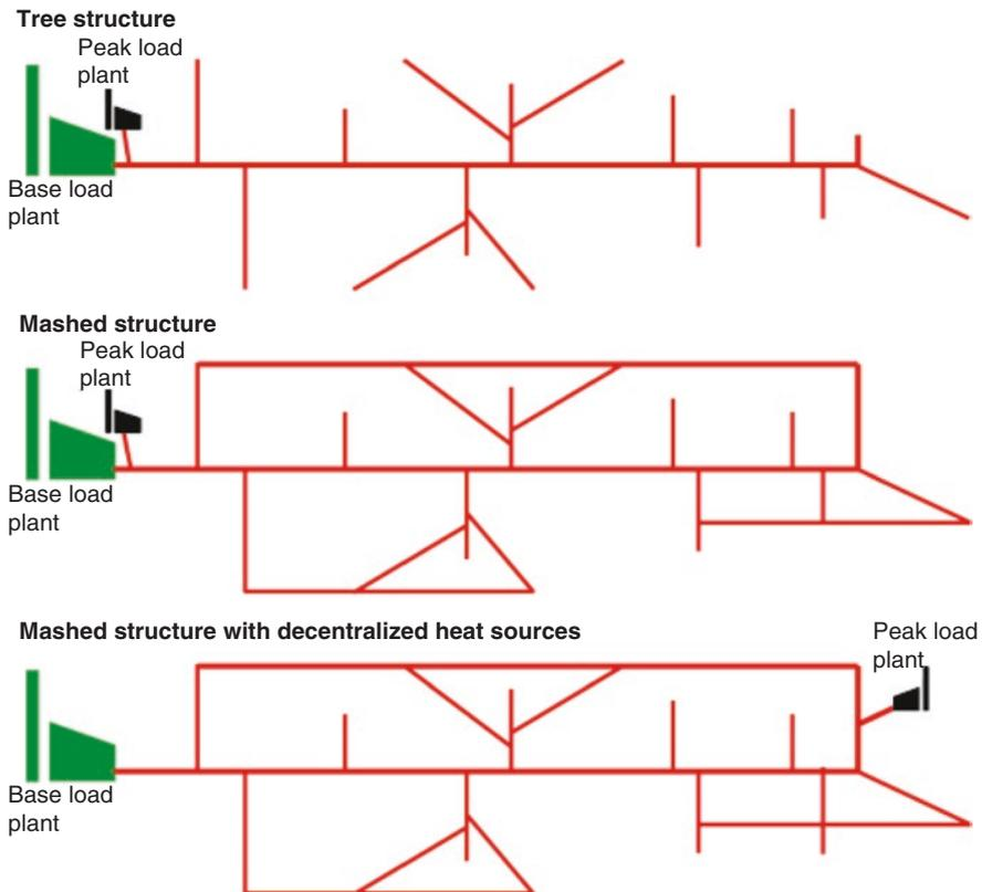
Fig. 7.12 Resilient heat supply strategies using local backup or a meshed network structure
