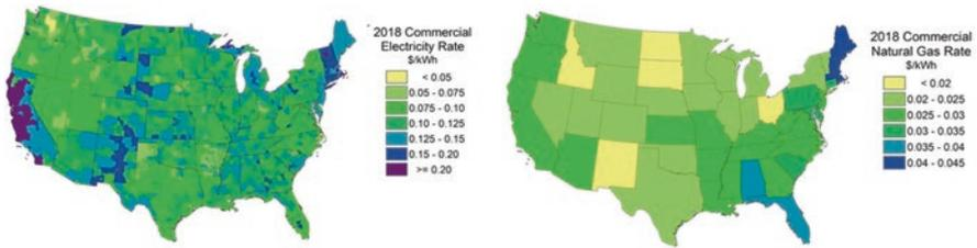
**Fig. G.2** For comparison to the calculated LCOE maps, these maps show electric rates (left) varying from less than \$0.05/kWh in the Pacific Northwest to \$0.20/kWh in California and natural gas rates (right) that vary from <0.02/kWh (thermal) in the Dakotas to \$0.045/kWh thermal in the Northeastern United States.
