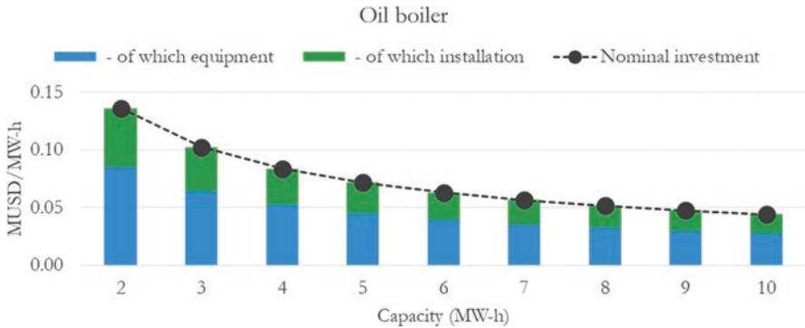
**Fig. F.44** Nominal investment by capacity for an oil boiler
