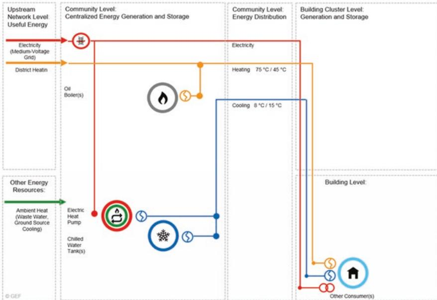
Fig. B.3 Energy system architecture for case study on district cooling in Taarby, Denmark
