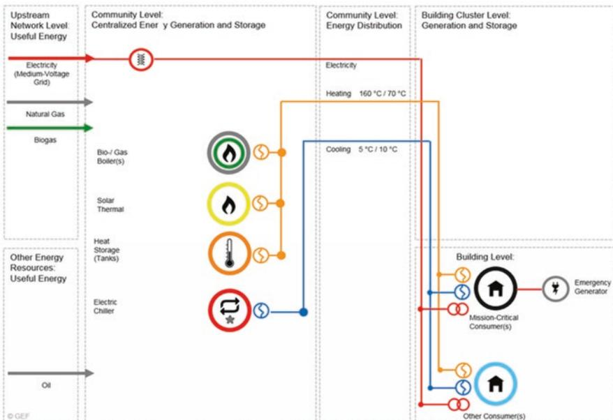
Fig. B.4 Energy system architecture for case study on University of California, Davis, United States
