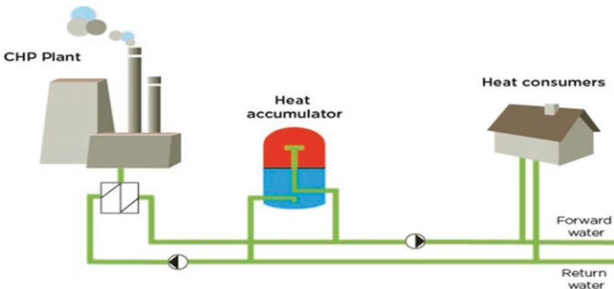
**Fig. F.51** The pressureless directly connected tank operates in a simple way. The tank compensates automatically for the difference in flow in the supply pump and the production pump
