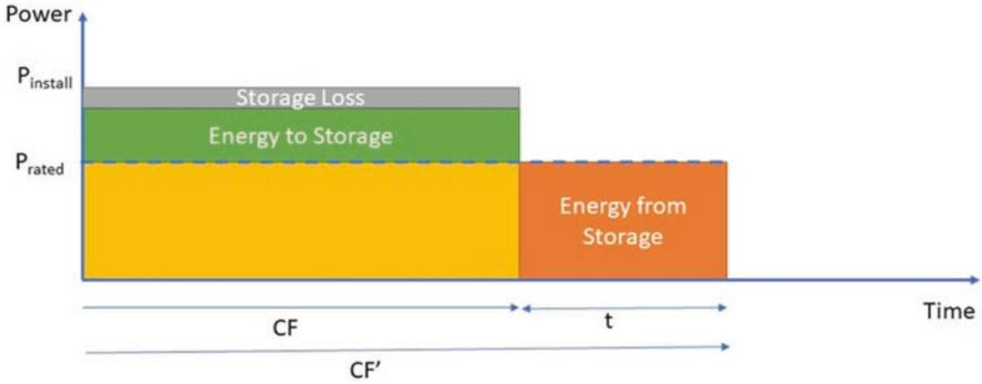
**Fig. G.1** Graphical representation of power into storage due to  $P_{\text{install}} > P_{\text{rated}}$  and resulting hours of energy storage,  $t$
