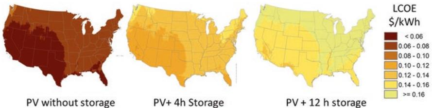
**Fig. G.3** LCOE across the Continental United States (CONUS) for photovoltaic systems including 4 hours and 12 hours of battery storage. Costs in sunny areas are on the order of \$0.06/kWh without storage and up to \$0.16/kWh in less sunny areas with 12 hours of battery storage
