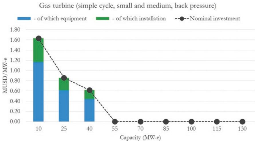
**Fig. F.7** Nominal investment for a simple cycle gas turbine (small and medium back-pressure)
