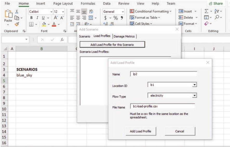
Fig. H.30 Adding the load profile for hurricane
