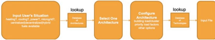
**Fig. 8.2** Architecture selection process
