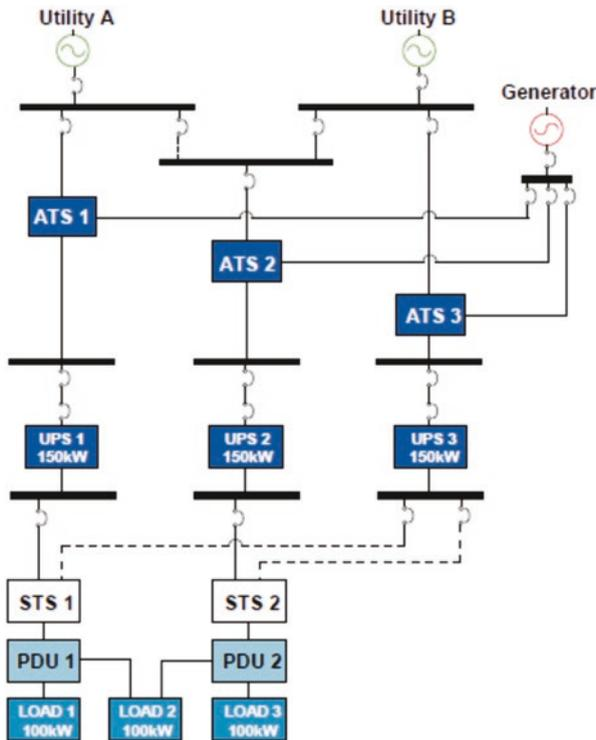
**Fig. C.6** Distributed redundant UPS configuration with static transfer switch (STS). (McCarthy and Avelar 2016)
