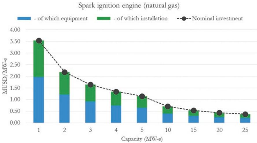
Fig. F.2 Nominal investment by capacity for a spark ignition engine using natural gas
