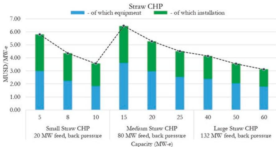
**Fig. F.11** Nominal investment for straw CHP (20, 80, 132 MW feed, back-pressure)
