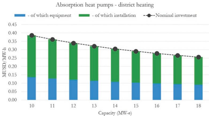
**Fig. F.49** Nominal investment absorption heat pumps—two-stage hot water
