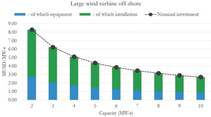
Fig. F.24 Nominal investment for large offshore wind turbine
