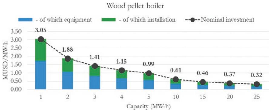
**Fig. F.38** Nominal investment by capacity for a wood pellet boiler
