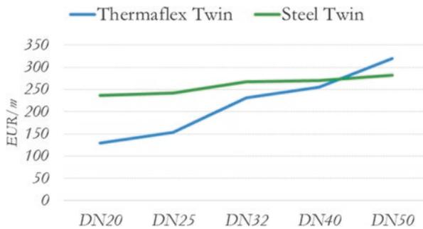
**Fig. F.84** Cost comparison between Thermaflex Twin and Steel Twin
