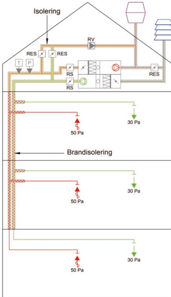
Fig. F.70 Central ventilation with heat recovery
