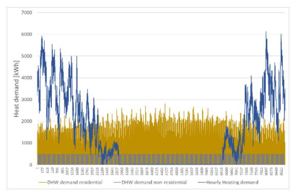
Figure 5-30. Simulation of the heating and domestic hot water (DHW) demand for the case study.
