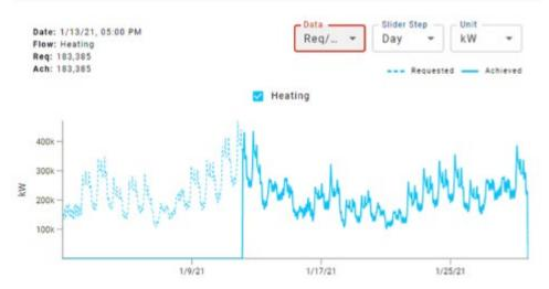
Figure 5-15. Boiler Plant Loads Requested vs. achieved.
