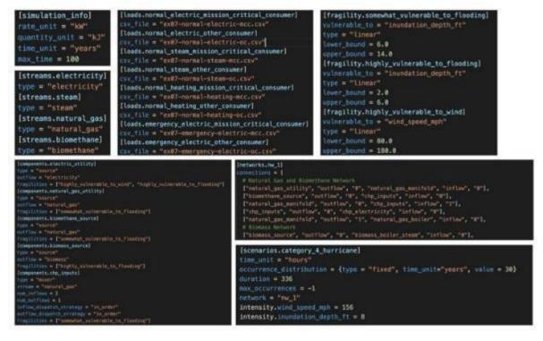
Figure 3-2. An example of a TOML file that the ERIN tool uses as an input in a standalone application.
