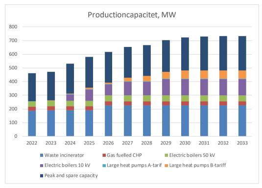
Figure 5-37. Heat production capacity.
