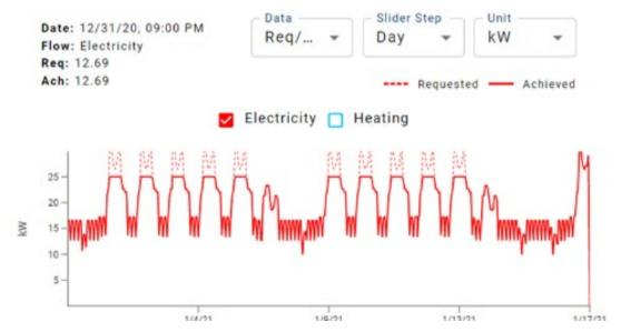
Figure 5-14. Facility LMCN cannot get enough power to cover peaks.
