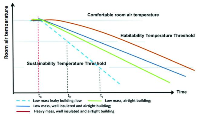
**Figure 4** Notional example of temperature decay rate for different types of building envelope: comfortable level  $t_o$ , habitability  $t_h$  and sustainability  $t_s$  temperature thresholds.
