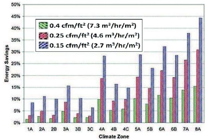
**Figure 6** Percent annual energy savings in a barracks building due to airtightness improvement for U.S. climate zones (Zhivov et al. 2014).
