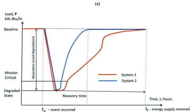
**Figure 3** Two systems with different levels of resilience: (a) different robustness and (b) different recovery time (Zhivov et al. 2021).
