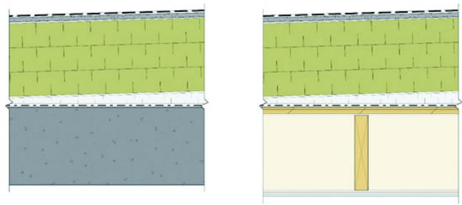
**Figure 7** Conventional roof assembly on a concrete structure (left) and on a wood structure (right). From exterior (top) to interior (bottom) these assemblies include roof membrane, cover board, insulation, tapered insulation, air and vapor control membrane, and structure.
