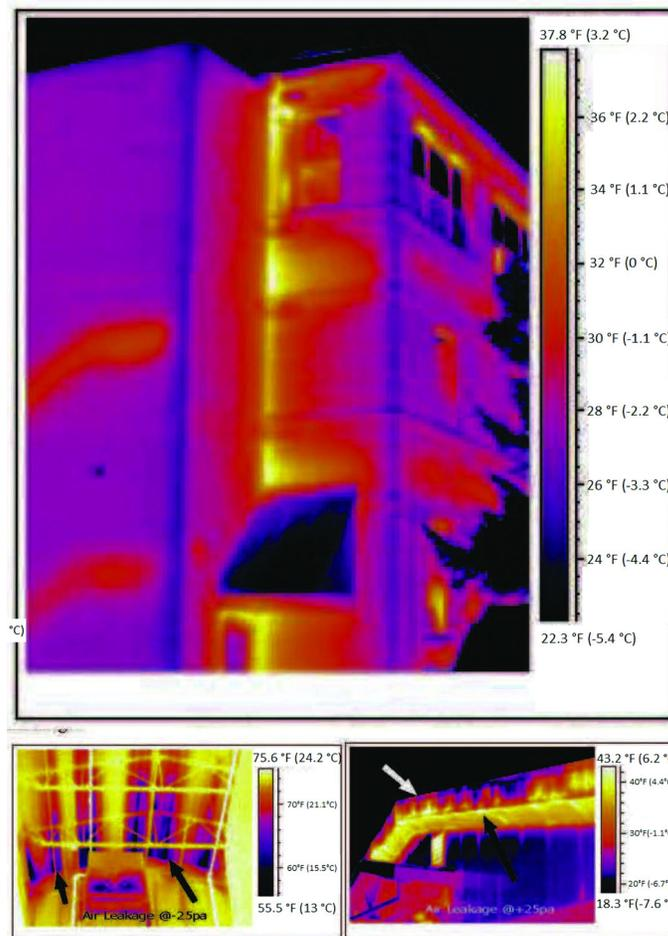
**Figure 5** Infrared thermographic image of typical thermal bridge in cold climates; Bottom: Infrared (IR) Images of air leakage at roof-to-rake wall joints. The building was tested to achieve air leakage rate of 0.25 cfm/ft² at 75 Pa (3.5 m³/h/m² at 50 Pa) (Leffel 2021).
