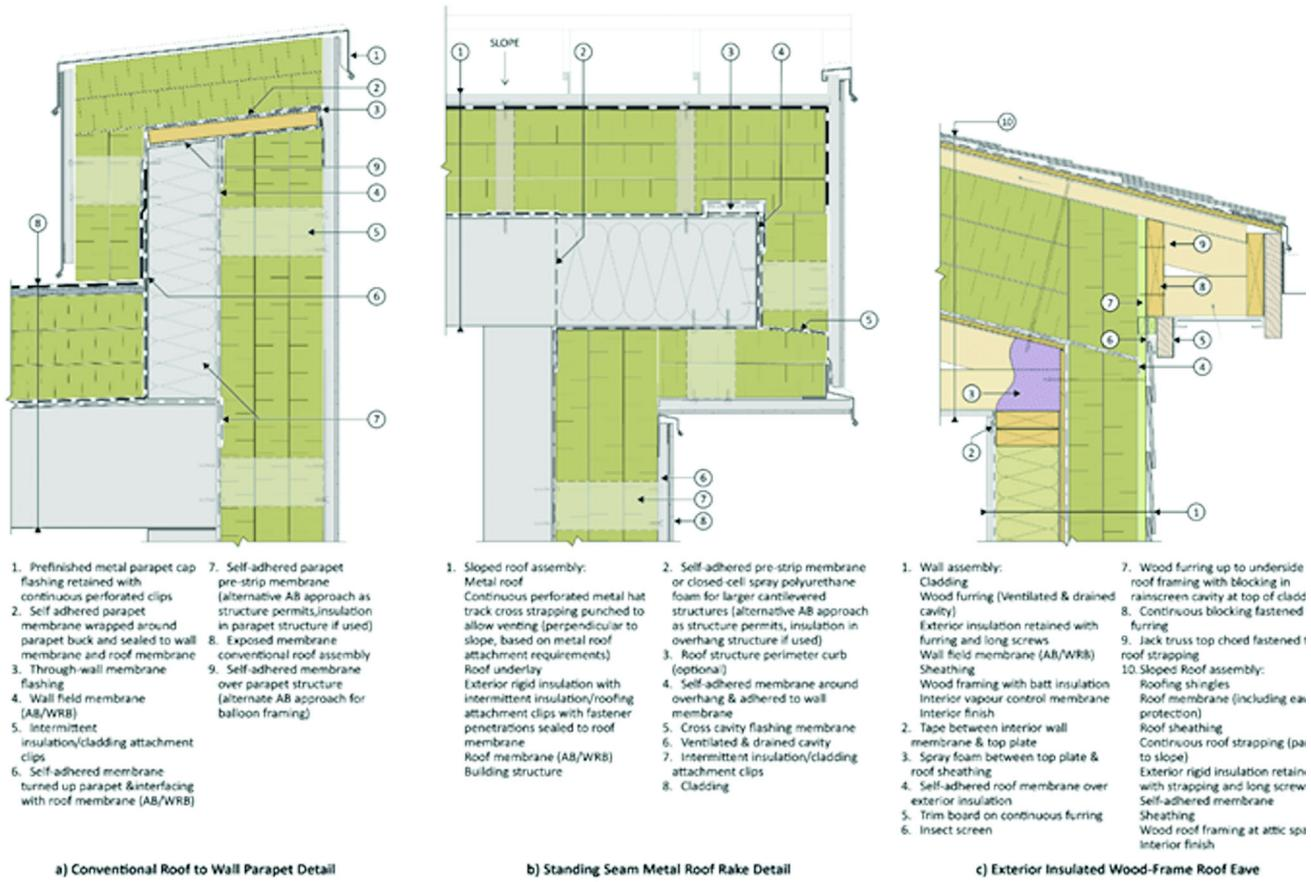
**Figure 11** Schematic roof-to-wall details showing key design elements for high-performance detailing, (a) conventional roof-to-wall parapet detail, (b) standing seam metal roof rake detail, and (c) exterior insulated wood-frame roof eave. In particular, note the continuity of control layers including the air barrier systems and the insulation in each of the details.
