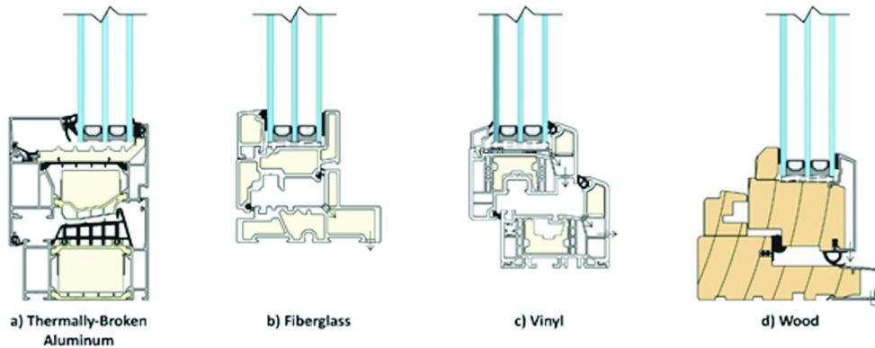
**Figure 9** High thermal performance window frame types, (a) thermally broken aluminum, (b), fiberglass, (c) vinyl, and (d) wood.
